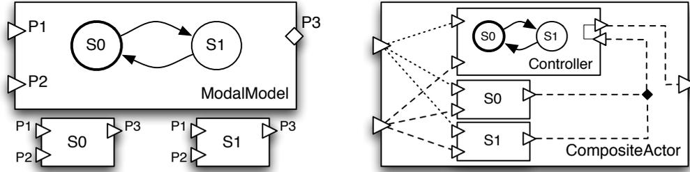
Figure 3: A modal model with 2 states and its equivalent representation as a composite actor.  $S0$  and  $S1$  are states, diamonds are input/output ports, and a solid line in the right-hand side means a coupled input/output ports.
