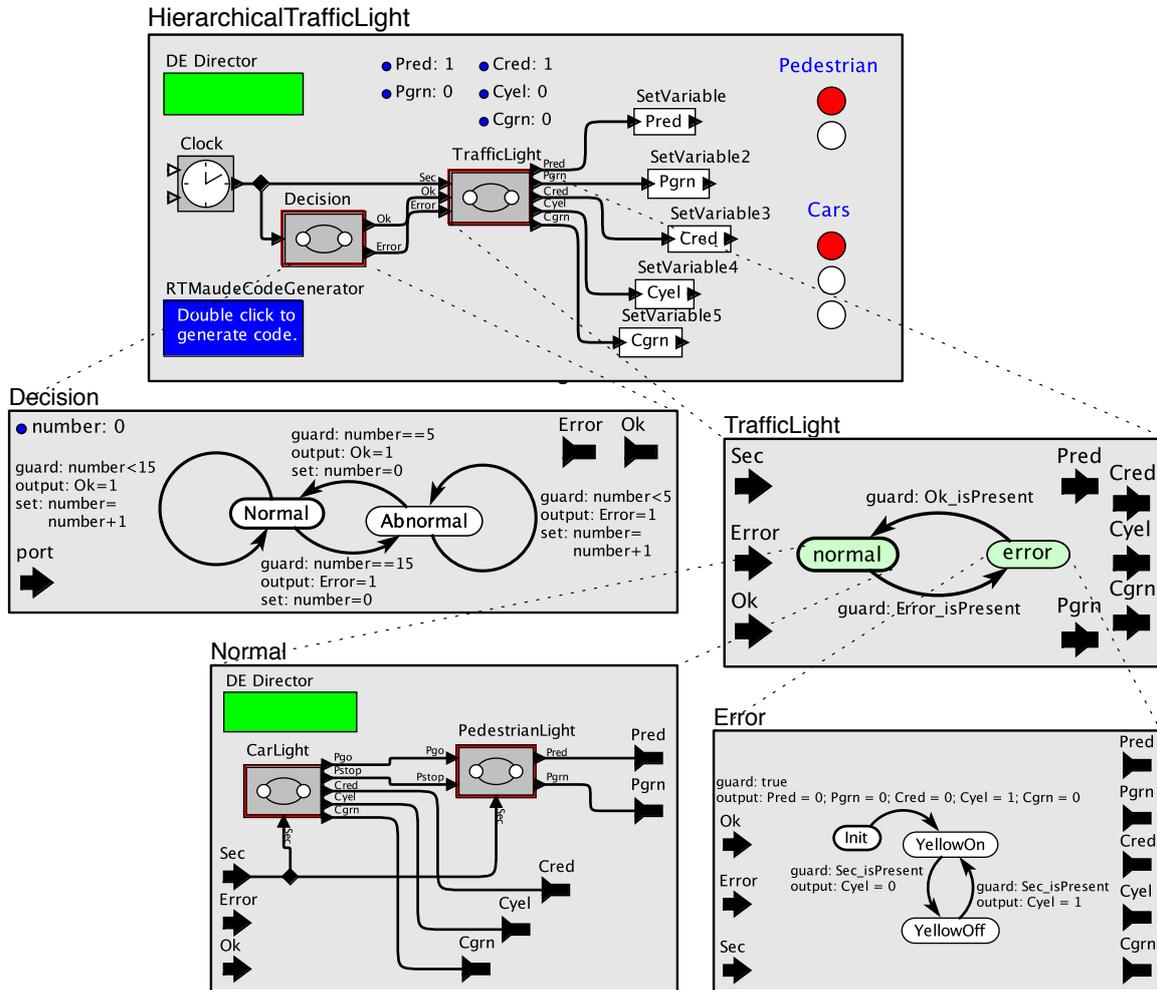
Figure 9: A hierarchical fault-tolerant traffic light system.
